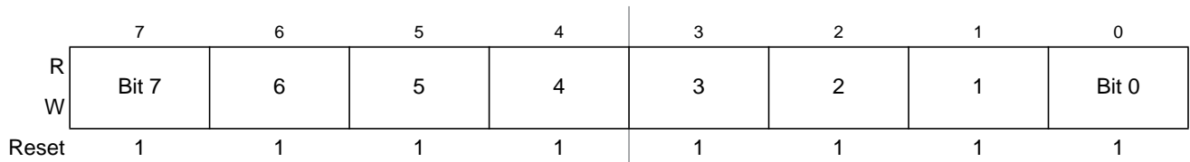
Figure 12-30. PWM Channel Duty Registers (PWMDTY3)
