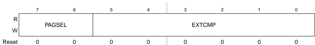
Figure 16-19. Debug Comparator B Extended Register (DBGCBX)
