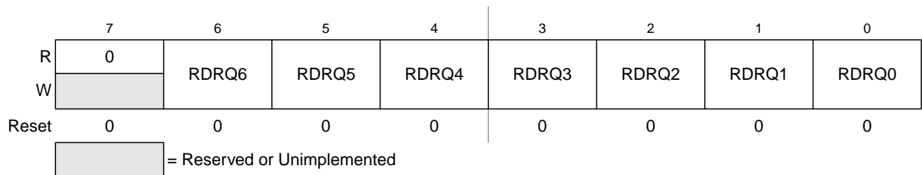
Figure 3-26. Port Q Reduced Drive Register (RDRQ)
